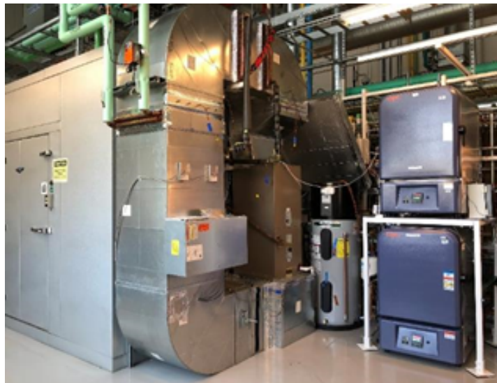
Figure 2. Hardware installed in the SPL for HIL experiment. The grey chamber on the left contains the condenser with the air handler and duct loop next to it. The top blue chamber on the right houses the thermostat.
