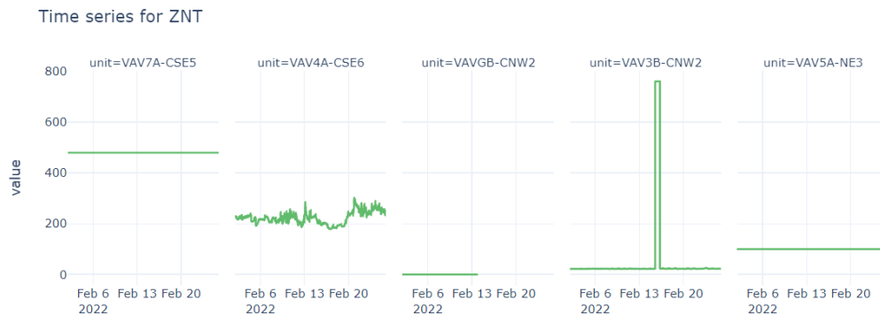
Figure 5. Time series plot showing top five most anomalous zone temperature readings.
