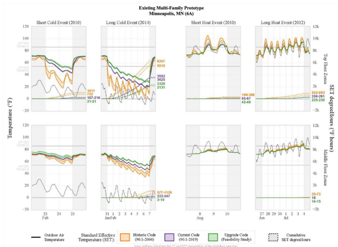
Figure 4. Exposure analysis results for Minneapolis existing multi-family existing prototype during a long heat and cold event. The feasibility study reflects a similar upgrade package to that of PHIUS.
