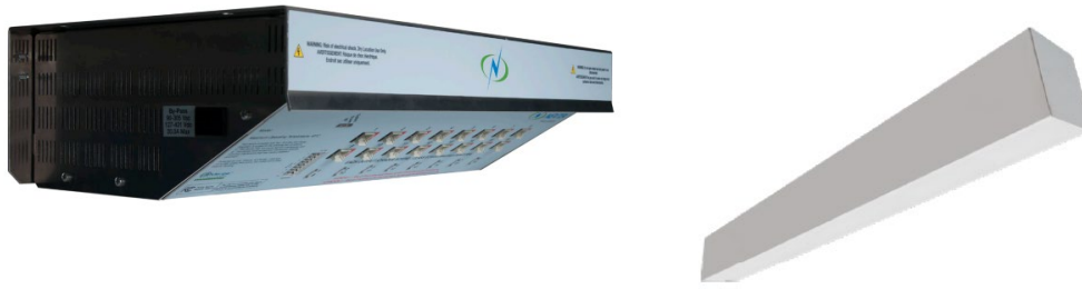
The Nextek Power Hub Driver (left) is a low voltage DC distribution system that converts 380VDC power to 24VDC to plug in Lamar DC lighting (right).
