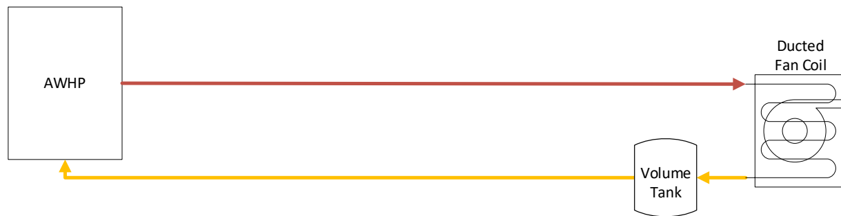
Figure 6. Ducted fan coil hydronic system schematic.
