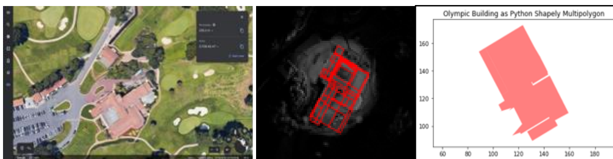
Figure 4. Left: An aerial view of the of Club House Building as seen on Google Earth; Center: an intermediate output in the machine learning process to extract building footprint; Right: ML-derived final footprint output. Note: Coordinates are transposed in plotting, and not visualized in the same orientation.
