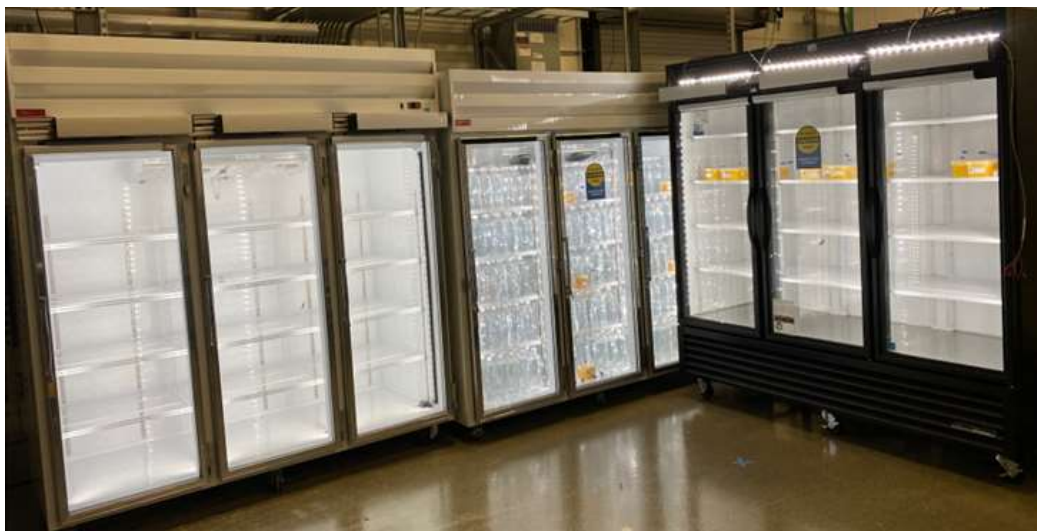
Figure 2. Image of the three refrigerator cases outside the environmental chamber. (Left) EE case B, (center) baseline case, and (right) EE case A. All images/figures by NREL.
