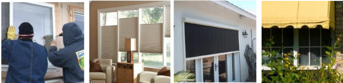
Figure 1. High Performance Window Attachments include (from left to right) exterior low-e storm windows, insulated cellular shades, exterior shades, and awnings. Sources: PNNL, AERC
