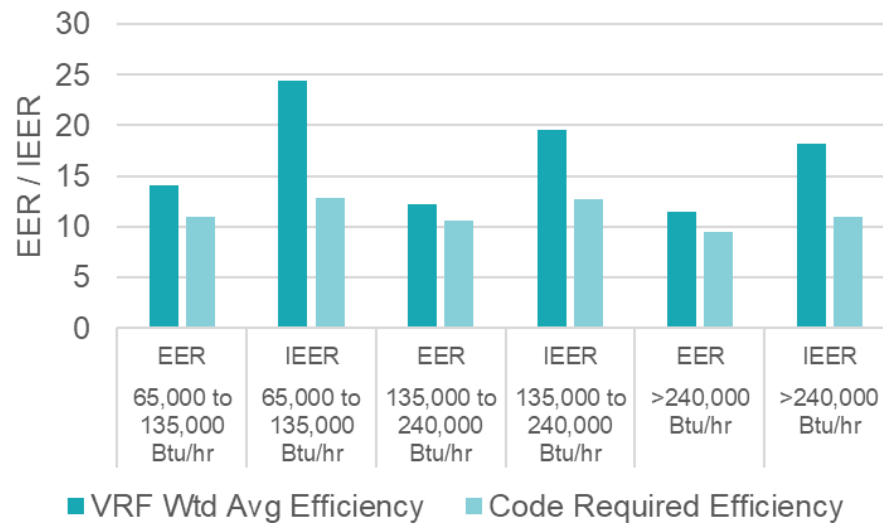
Figure 5: Comparison of regional weighted average VRF cooling energy efficiency ratio (EER) and integrated energy efficiency ratio (IEER) to code minimum efficiency requirements (by equipment size).
