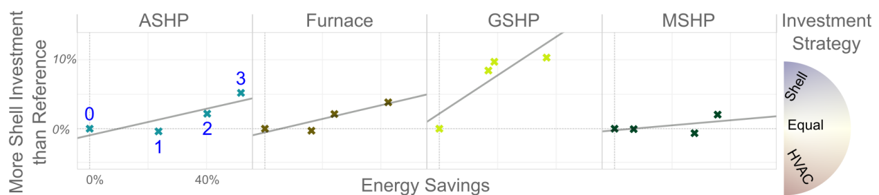
Figure 3. Shell investment ratio versus site energy savings. Source: NMR Group 2021, p.30.
