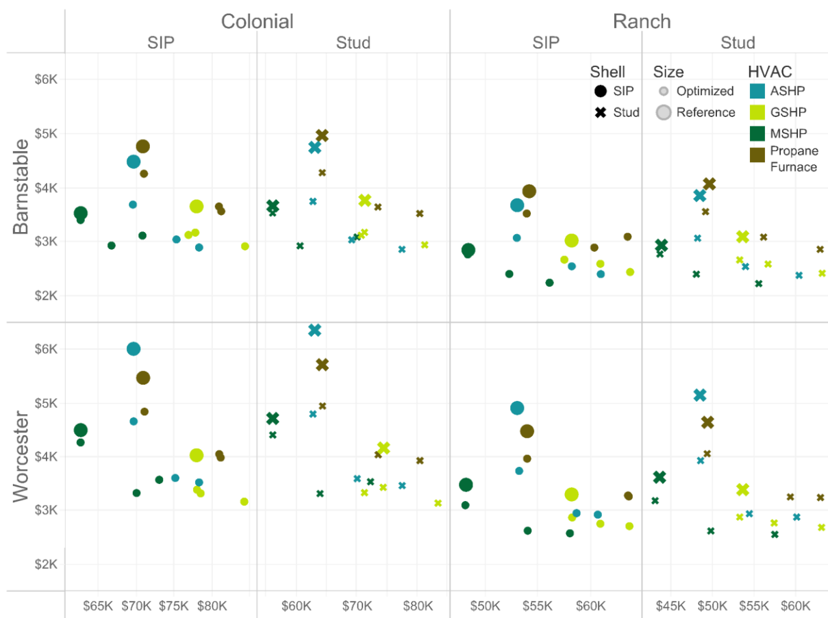
Figure 7. Construction versus annual utilities for propane and electrically heated packages. Source: NMR Group 2021, p. 121.
