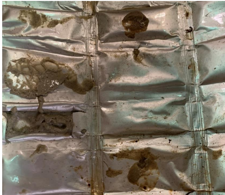
Figure 5. PCM mat with multiple leaks near scuff marks from Site 54.
