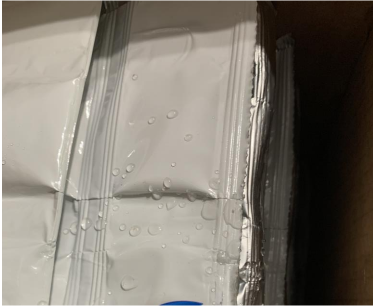
Figure 6. PCM mat with water accumulation but no apparent leaks.
