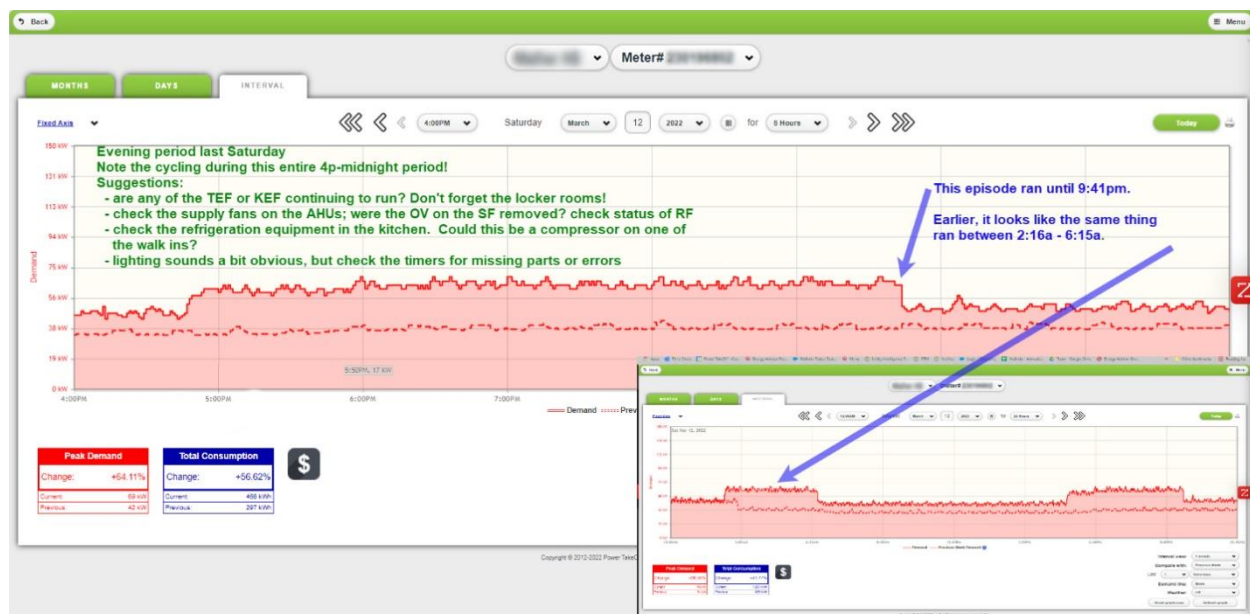
Figure 7. An image showing notes from investigating high weekend energy usage at High School a with the building engineer.
