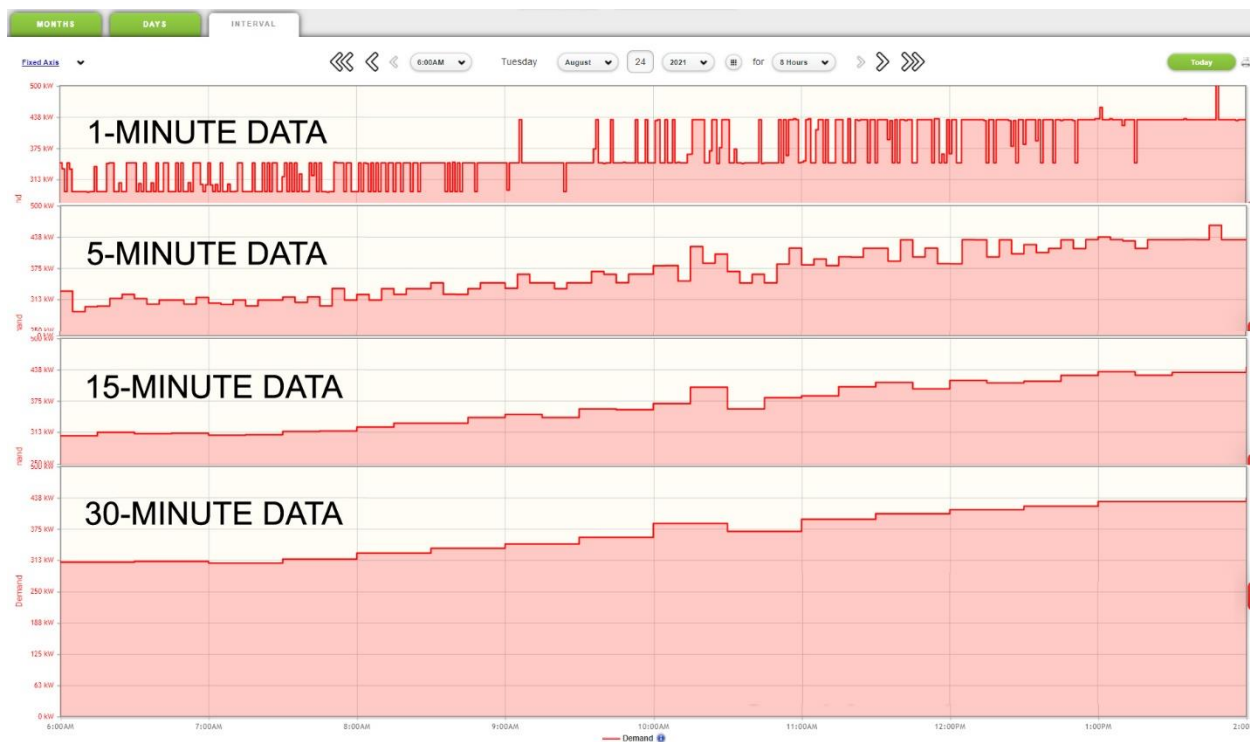
Figure 5. Early morning energy usage at Elementary School A showing difference in resolution of normal 30-minute interval data vs. 1-minute real-time data. The higher resolution real-time data enabled the identification of a malfunctioning freezer compressor.
