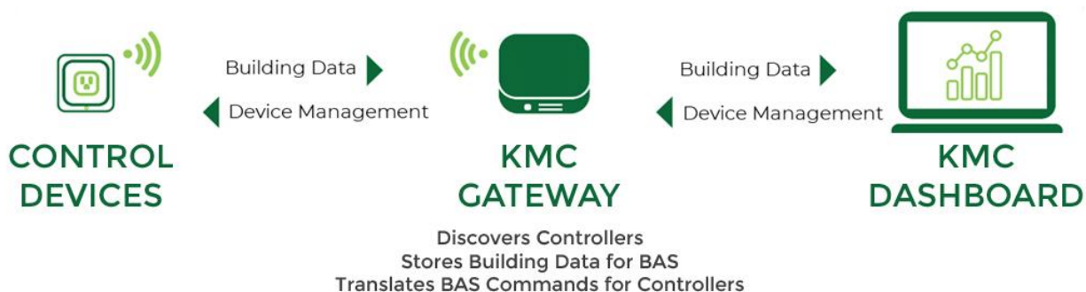
Figure 9. Plug load control device diagram and information flows.
