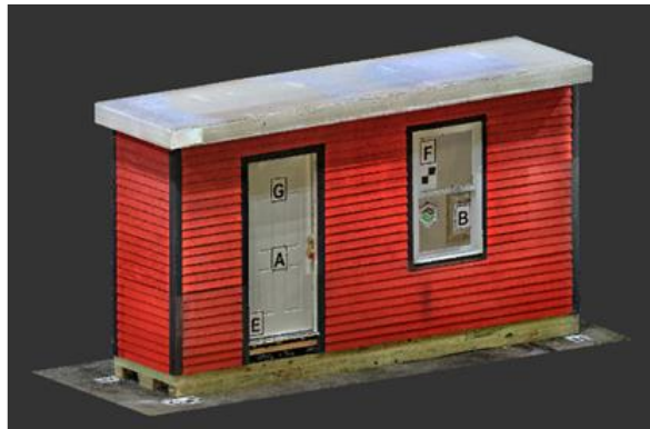
Figure 4. Point cloud scan of mock-up wall.
