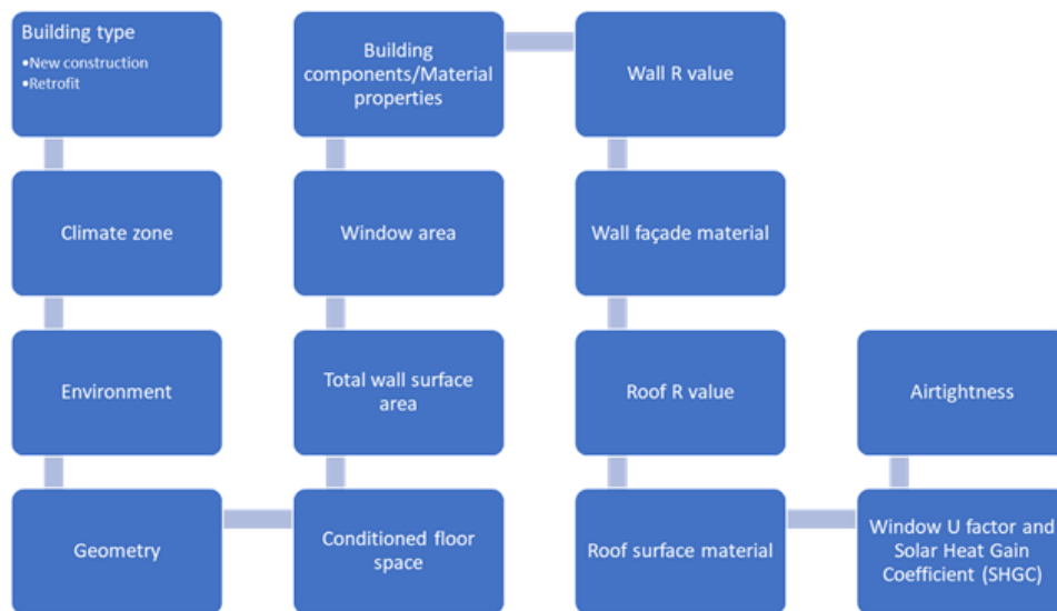
Figure 1. Process flow diagram that shows the inputs required by users to calculate the BEP metric.
