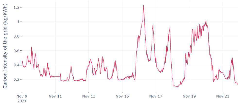
Figure 6. Carbon intensity of South Australia grid.
