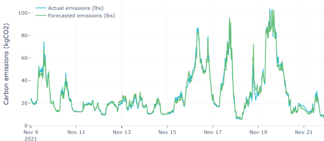
Figure 7. Actual and predicted emission profiles of a SA building.
