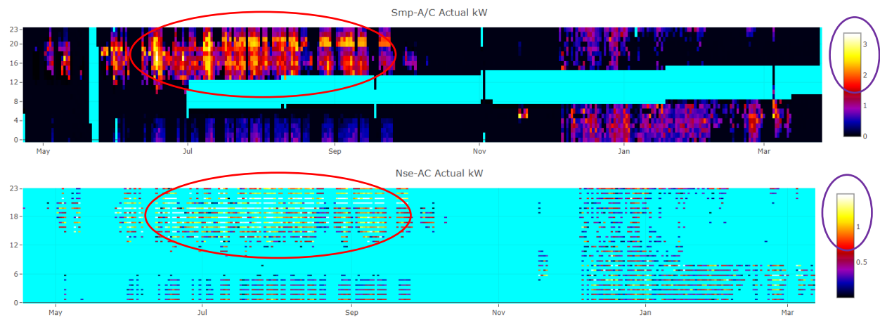
Figure 2. Site A: comparison of AC loads from measured CTs and Sense monitor showing agreement in timing of the load through the nearly identical pattern visible throughout the image and particularly apparent in the red circled section. The measurements were not in agreement in power magnitude shown in the scale on the right circled in purple. Notice that full scale for the CT measurement on top of the figure is 3 kW whereas full scale for the Sense monitor is 1.5 kW.
