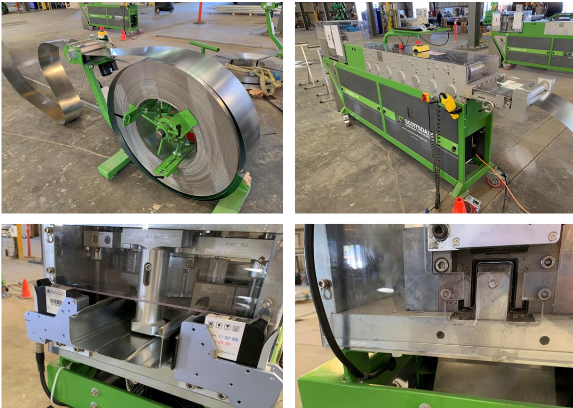
Figure 5. Top: Feedstock for an LGS machine. Bottom: LGS machines creating structural members with different cross-sections.
