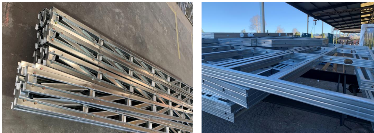
Figure 6. Truss and wall assemblies created using the LGS structural members prepared with the LGS machines.
