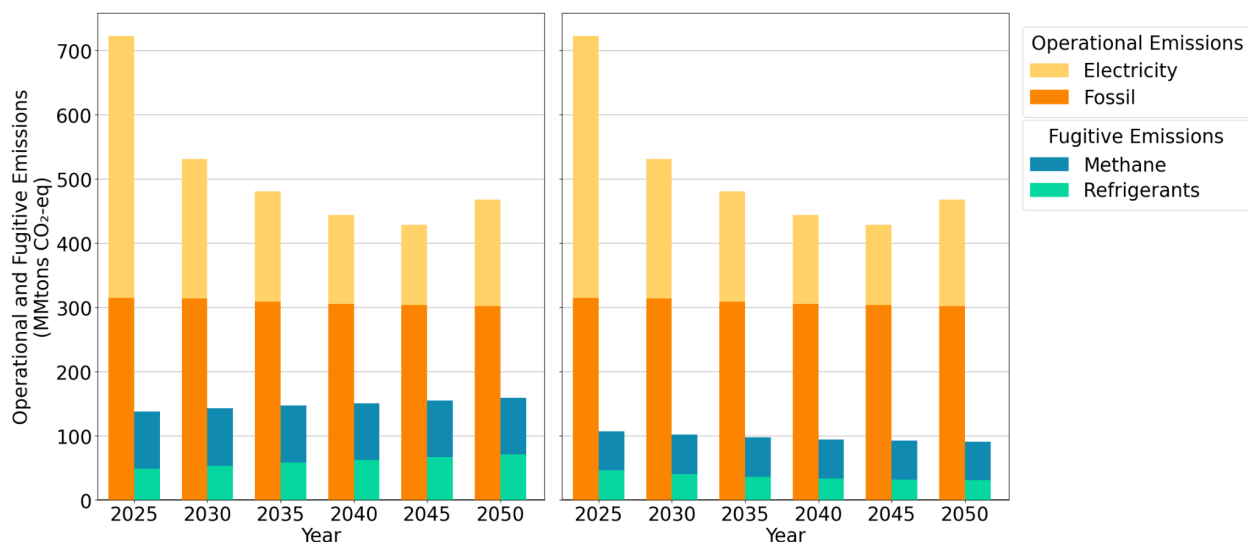
Figure 4. Worst-case (left panel) and best-case (right panel) estimates of total fugitive methane and refrigerant leakage emissions from U.S. residential building energy consumption from 2024-2050, compared to total operational emissions from direct on-site combustion of fossil fuels and indirect generation of electricity for residential building end uses, under a reference case.
