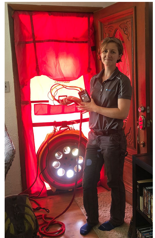
MACED Residential Energy Specialist Rachel Norton performs a blower door test on an Eastern Kentucky home. Source: Rachel Norton.
