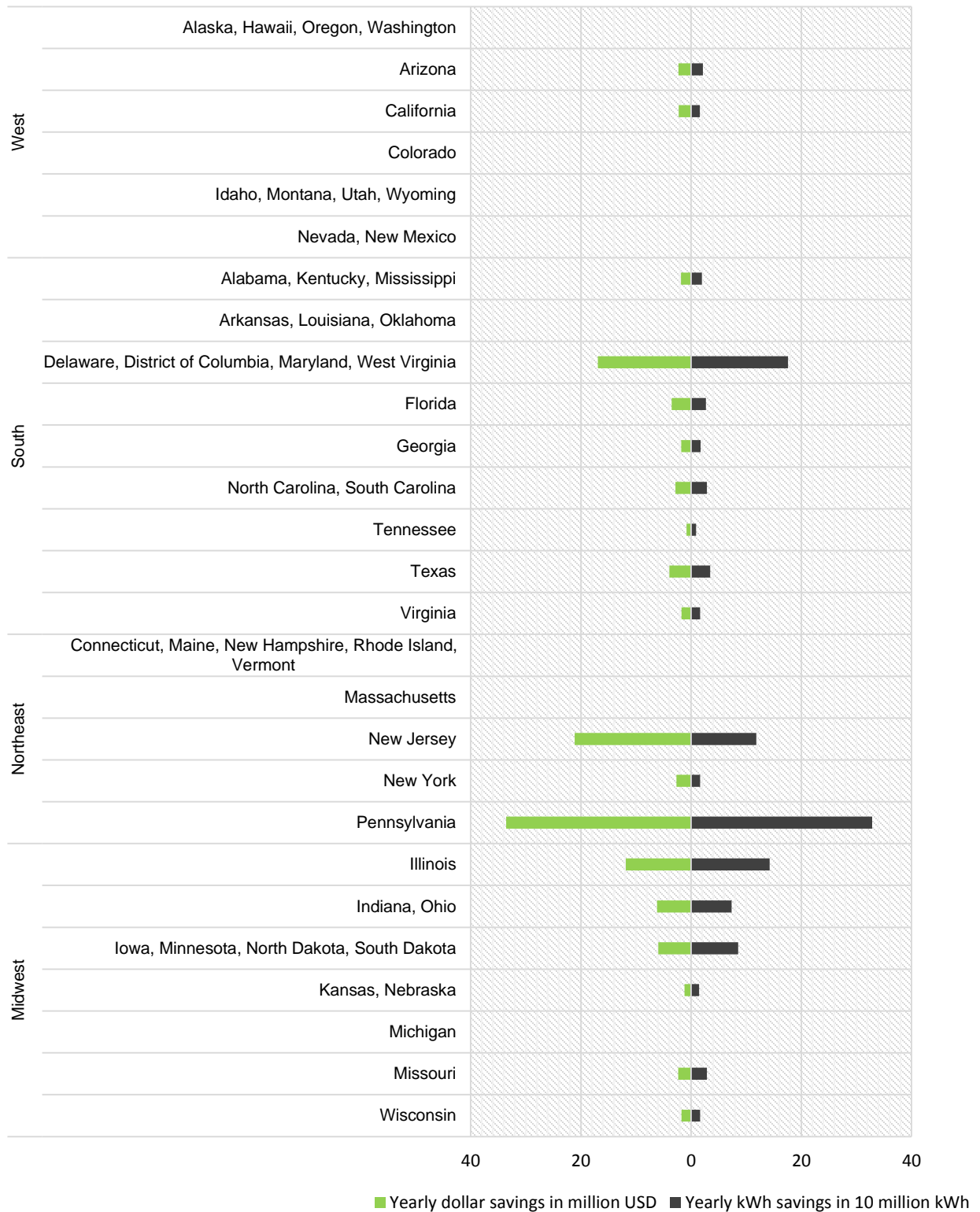
Figure 13. Estimated total annual energy and dollar savings by state or group of states for homes with electric baseboard and central air-conditioning. These figures are for single-family homes and multifamily buildings with two to four units per building, and apply the weighting factors in the RECS study. Source: ACEEE analysis of the detailed 2009 RECS data files.
