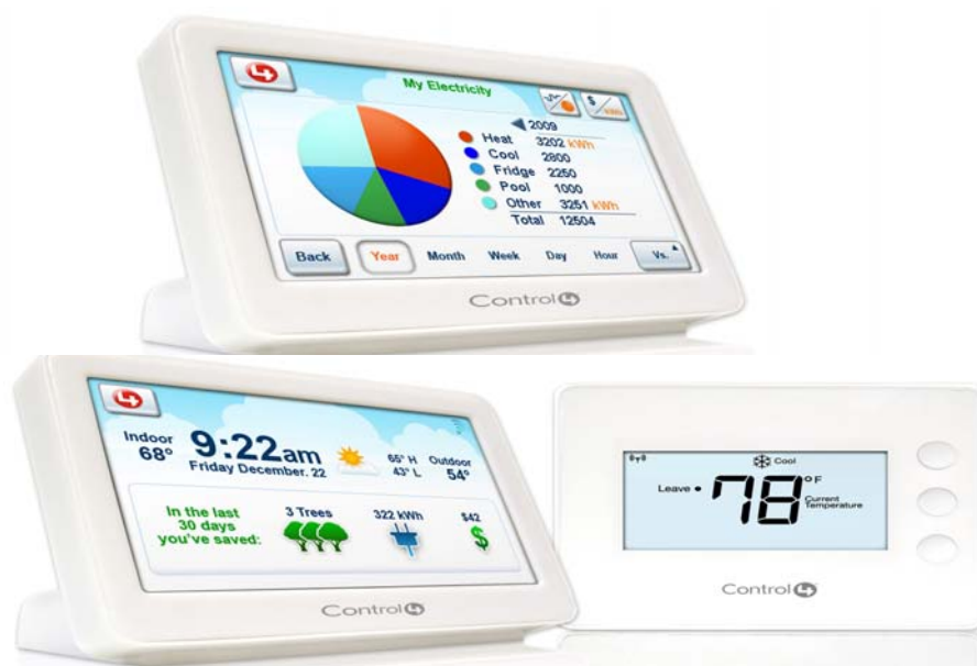
Figure 6: Control4 Touch Screen Whole-House Automation
