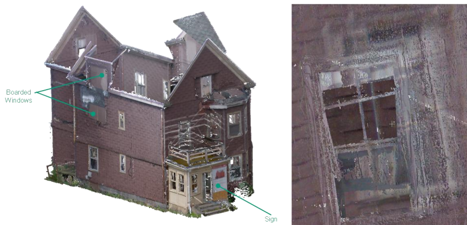
Figure 3. Example of a poorly scanned and registered building (left) resulting in indeterminate window location and geometry (right).
