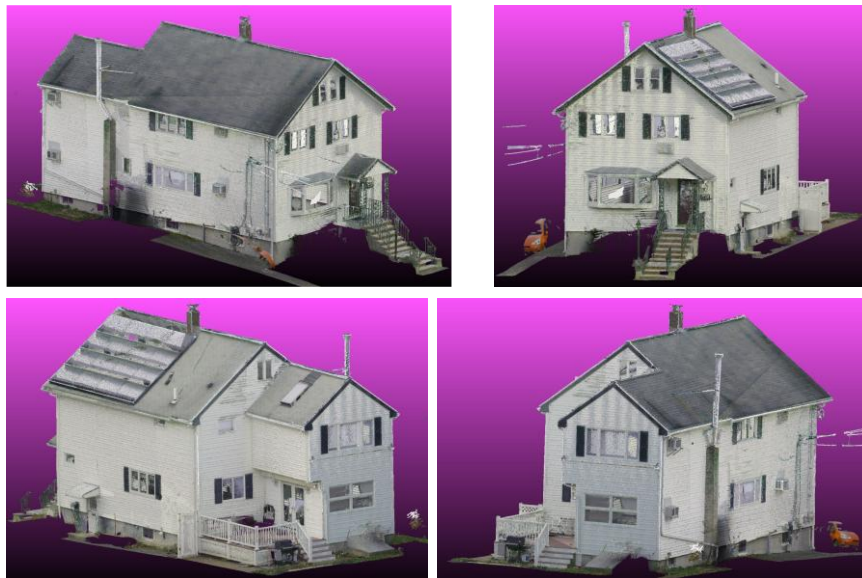
Figure 5. Example of a high-quality registered point cloud for a single-family building.
