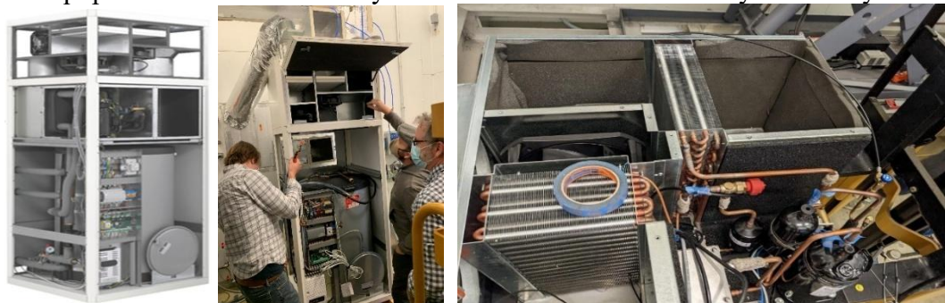
Figure 1: (Left) Diagram of the Systemair Genius product, (center) the system set up for testing in the Lab, and (right) the compact design of the heat pump module.
