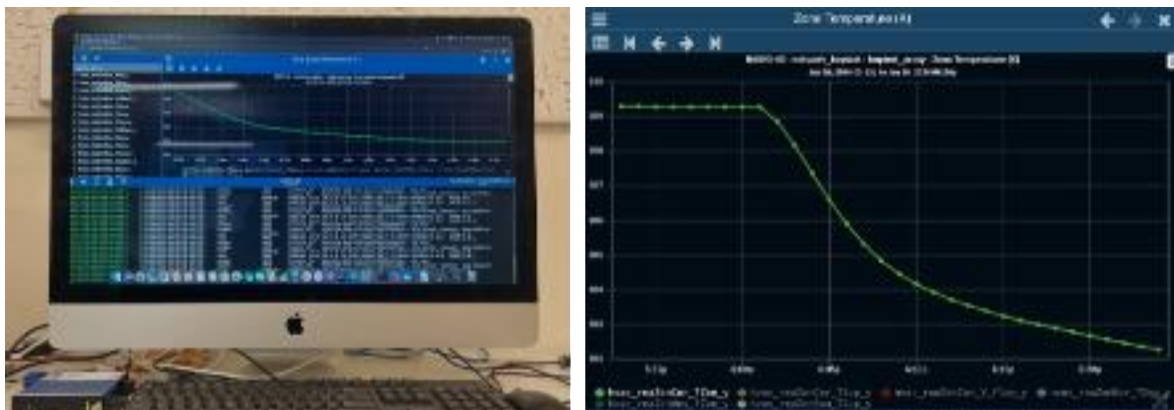
Figure 3: Image of case study. Left, BAS connected to a desktop running BOPTEST and BACnet network. The top window shows the BAS interface, the bottom window shows BOPTEST simulating a damper stuck fully open. Right, BAS trend showing the zone temperature rapidly cooling due to the stuck damper fault beginning at 6:00 pm.
