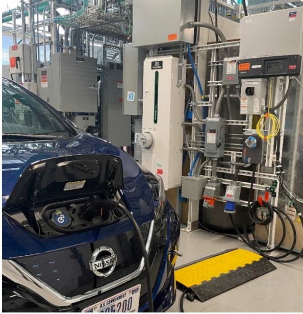
Figure 1. Laboratory setup showing Schneider Electric Panel, EV and EVSE, and PV inverter.
