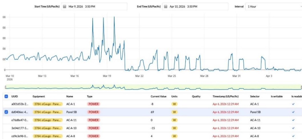
Figure 6. Submeter with 4 representative HVAC units showing reduction in HVAC loads.
