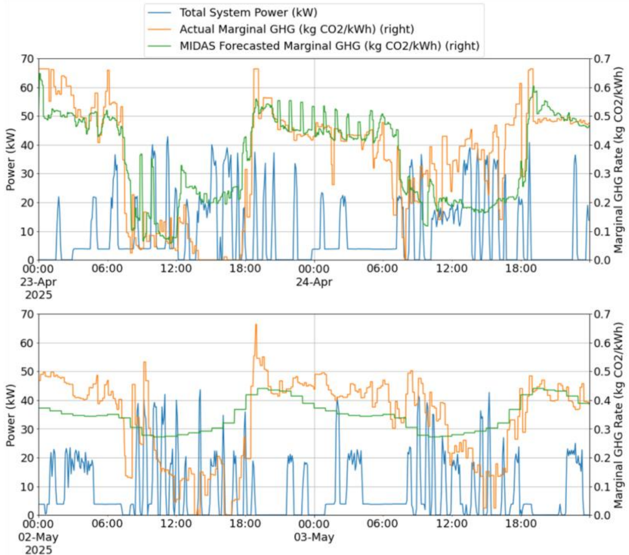
Figure 7. Subset of Gilroy GHG optimization testing using MIDAS. The upper plot represents two days where the forecast appeared to be correct. The lower plot represents a simplified forecast provided by the MIDAS server. This includes muted peaks and valleys compared to both actual marginal emissions factors and typical forecasts.
