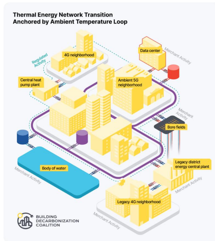
Figure 1. Fifth generation thermal energy network diagram
