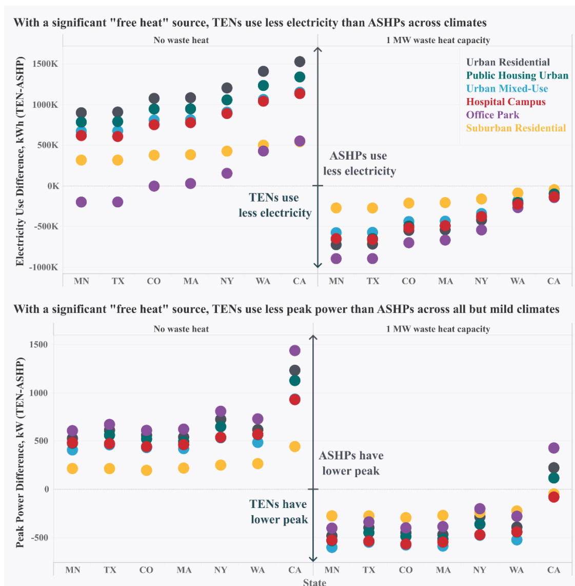
Figure 3. Distribution of electricity use (top) and peak power (bottom) differences between TENs and ASHPs across simulations
