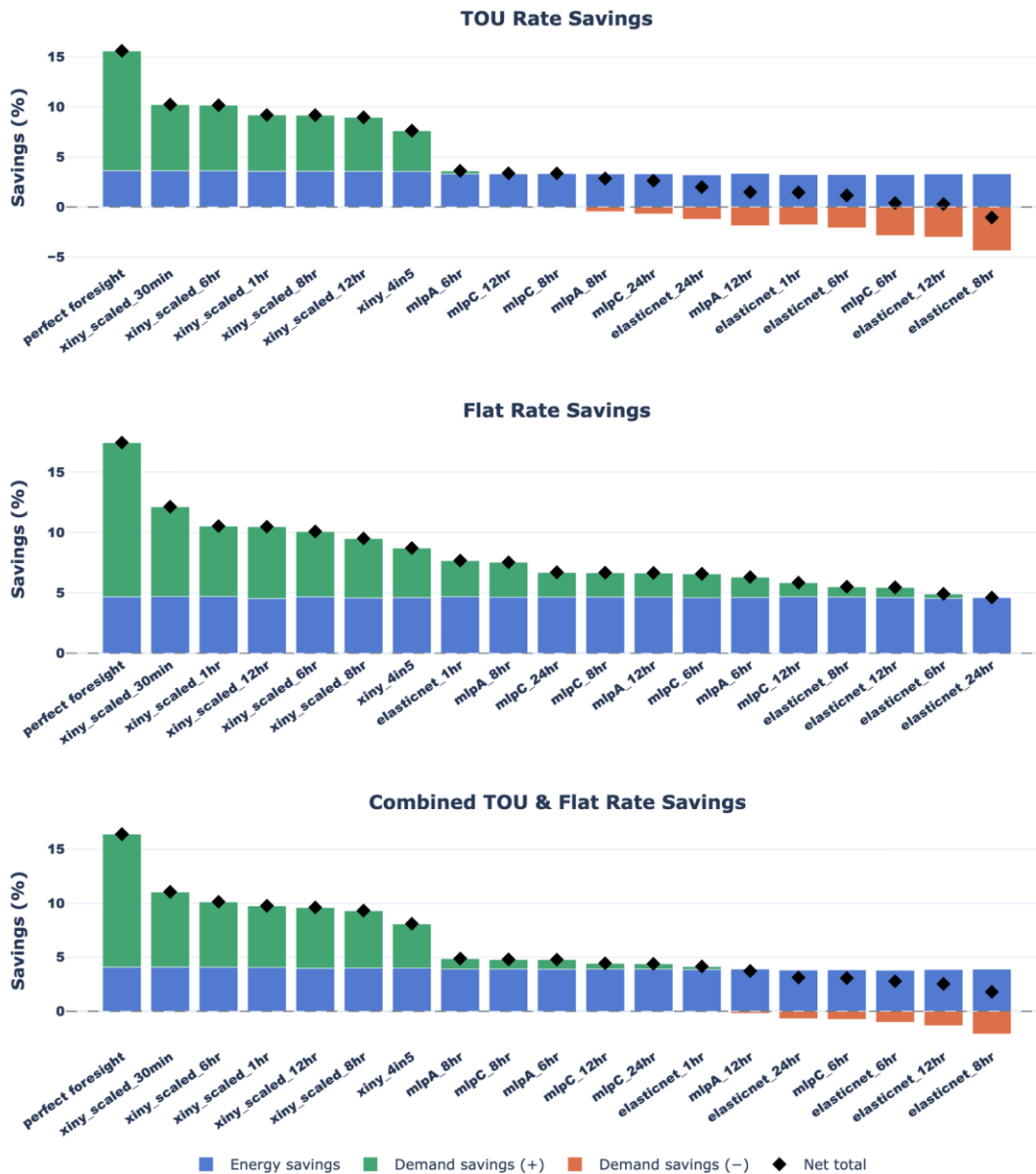
Figure 4. Savings percentage from the economic dispatch model for an electricity tariff with TOU rates (top), an electricity tariff with flat rates (middle), and the combination of savings from both rate structures representing a portfolio of buildings with customers on both tariffs (bottom). Perfect foresight represents results from the economic dispatch model with full information about future building load, and all other bars represent the results of the economic dispatch models optimized to different forecasts.
