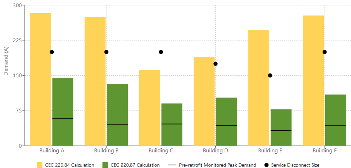
Figure 1: Full Electrification Calculated Electrical Load. The figure shows the difference between the results of NEC 220.84 and 220.87 when used to calculate the electrical load of 6 buildings fully electrified with the equipment specified in Table 2.
