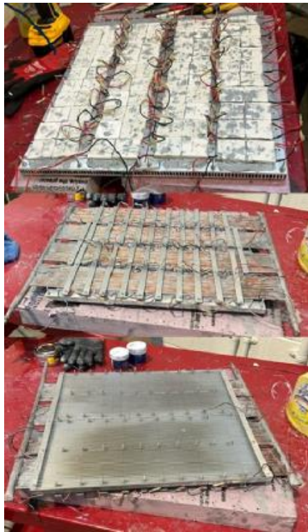
Figure 2. Fabrication process for the modular thermoelectric subcooler. Left: TE subcooler containing TE modules sandwiched between capillary tube bundles and fin base. Right: 24V direct current fans placed above the fin base.
