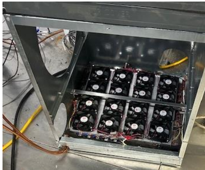
Figure 2. Fabrication process for the modular thermoelectric subcooler. Left: TE subcooler containing TE modules sandwiched between capillary tube bundles and fin base. Right: 24V direct current fans placed above the fin base.
