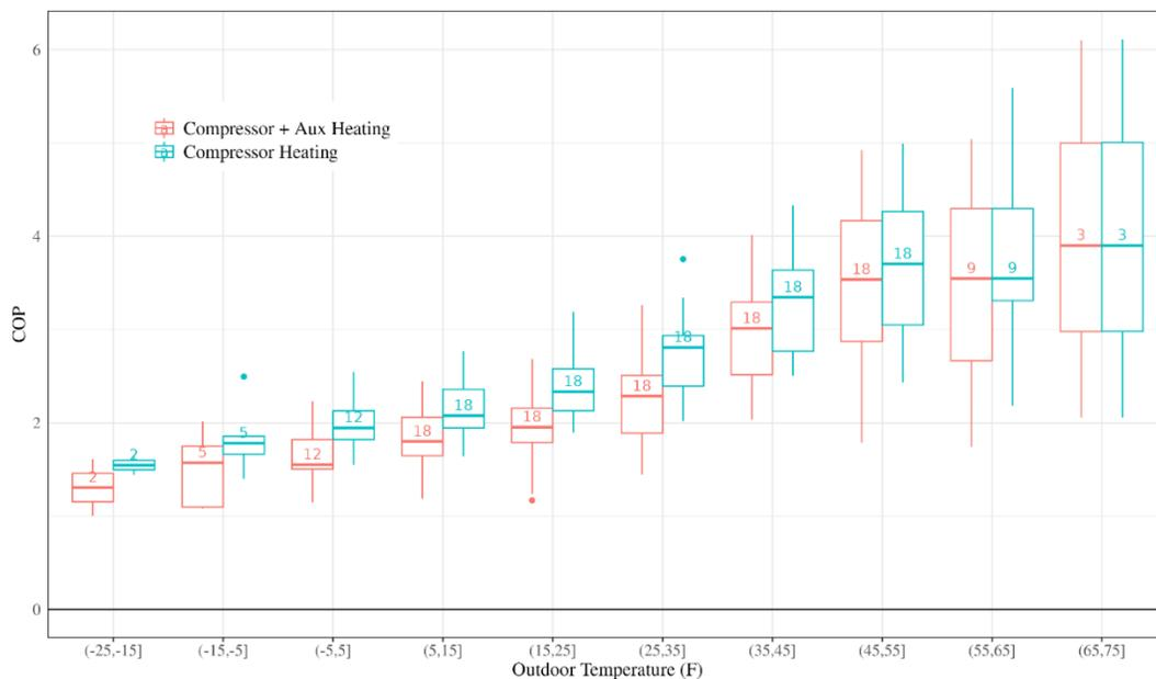
Figure 4. Heating COP by Outdoor Air Temperature Bin. The count of sites with data used for each boxplot is labeled within the box.
