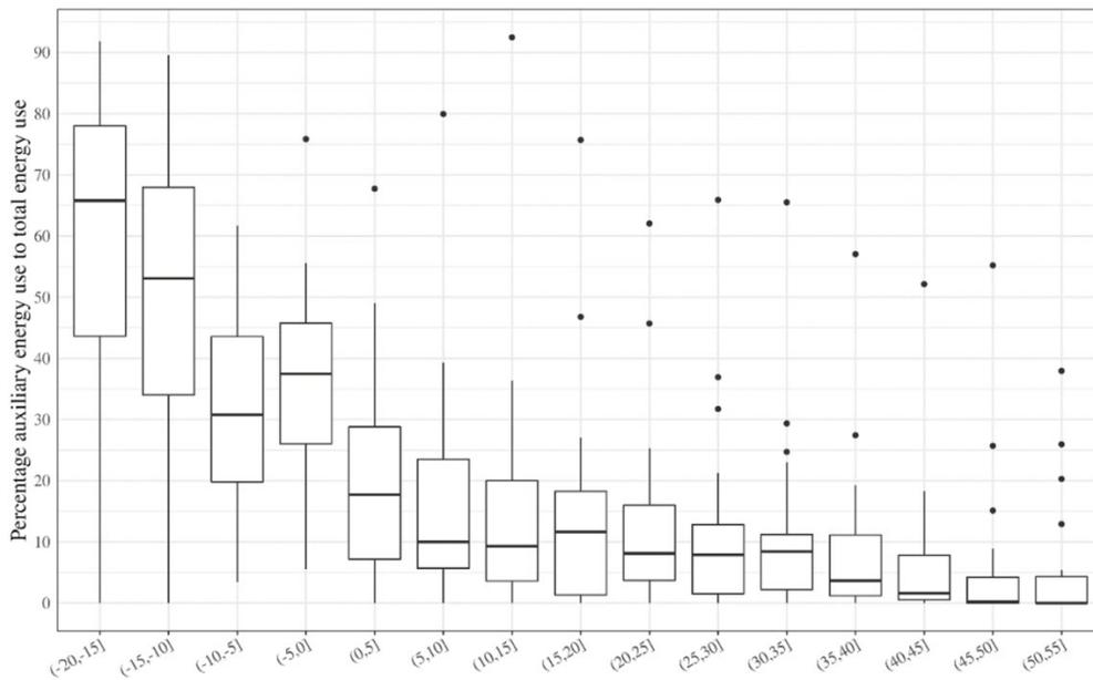
Figure 6. Auxiliary Heat Support by Outdoor Air Temperature Bin.
