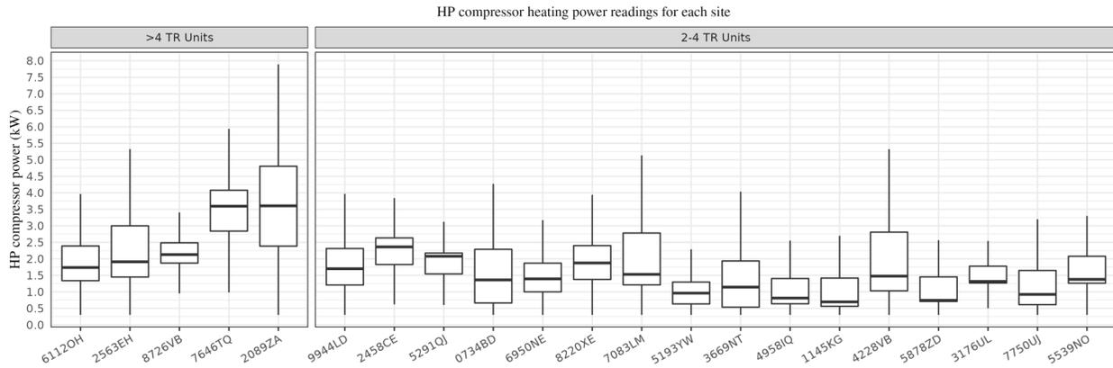
Figure 5. Compressor Power Categorized by Unit Size.
