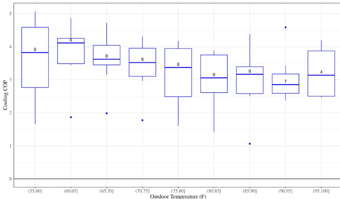
Figure 7. Cooling COP by Outdoor Air Temperature Bin. The count of sites with data used for each boxplot is labeled within each box.
