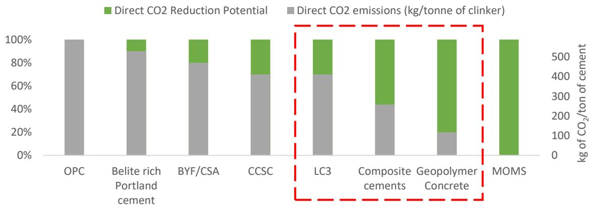
Figure 3: Emissions reduction potential of various low carbon alternative w.r.t OPC. Sources: (Scrivener, et al. 2018), (Hassan, Arif and Shariq 2019), (CII 2016), (Naqi and Jang 2019), (Sahu and Meyer 2020) , (The American Ceramic Society 2011)
