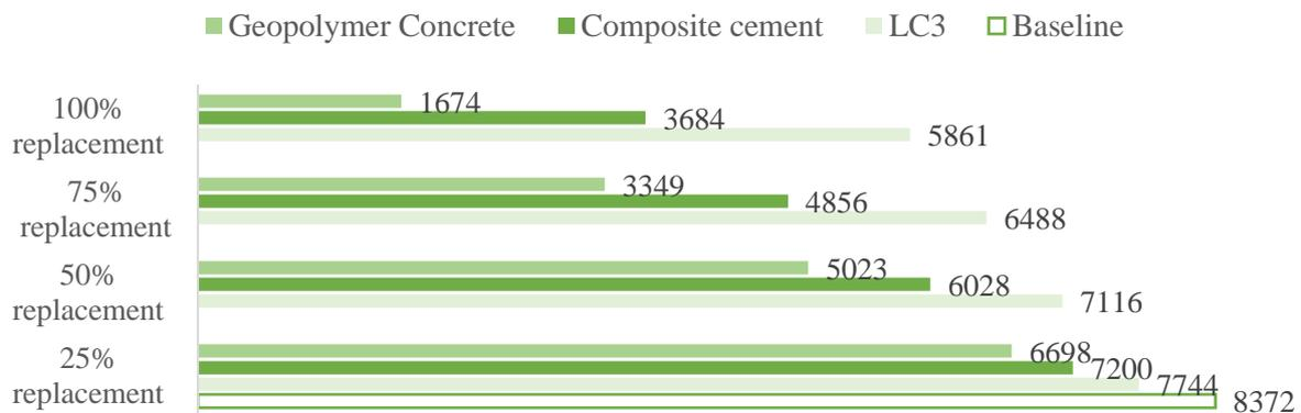
Figure 4: Reduction in GHG emissions in MtCO<sub>2</sub>/ton of cement by 2047- Supply-side interventions
