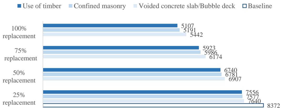
Figure 5: Reduction in GHG emissions in MtCO<sub>2</sub>/ton of cement by 2047- Demand-side interventions
