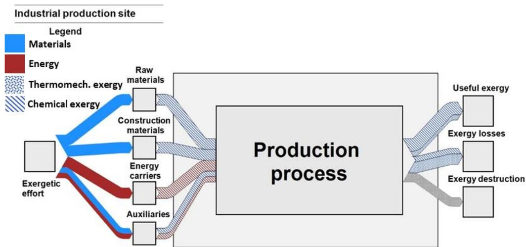
Figure 5: Sankey diagram of an exergetic analysis of an industrial production site (Own figure)
