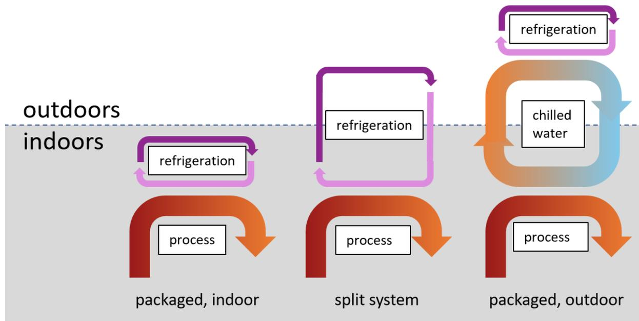
Figure 1. Three common system configurations using chillers: packaged indoor, split system, and packaged outdoor.
