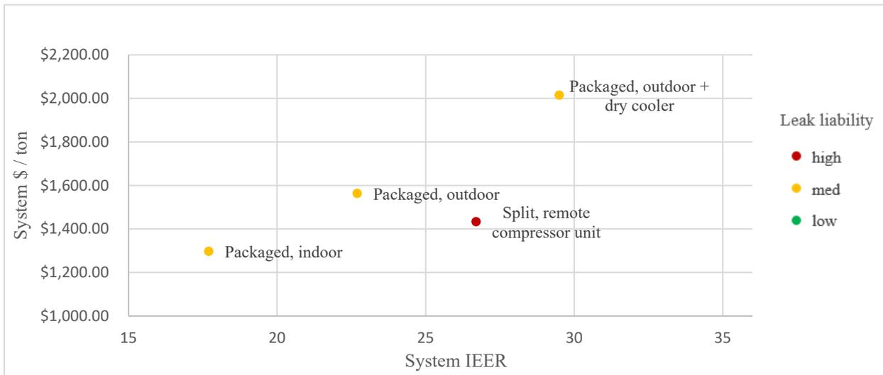
Figure 2. Process cooling system-integrated energy efficiency ratio as it related to pricing per ton of cooling. Pricing data is taken from projects between 2018 and 2020.
