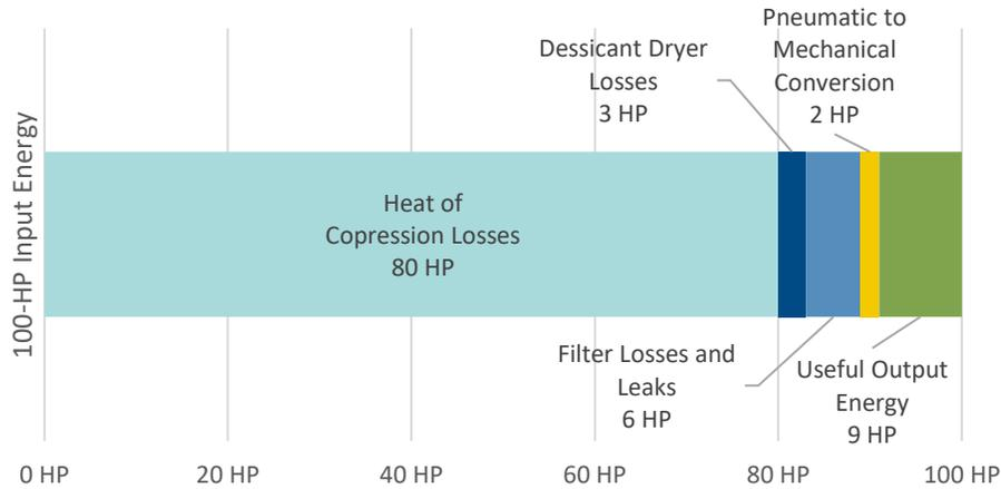
Figure 2. Relative breakdown of losses in a typical compressed air system assuming 100-hp of input energy. *Source:* CEATI, 2007.
