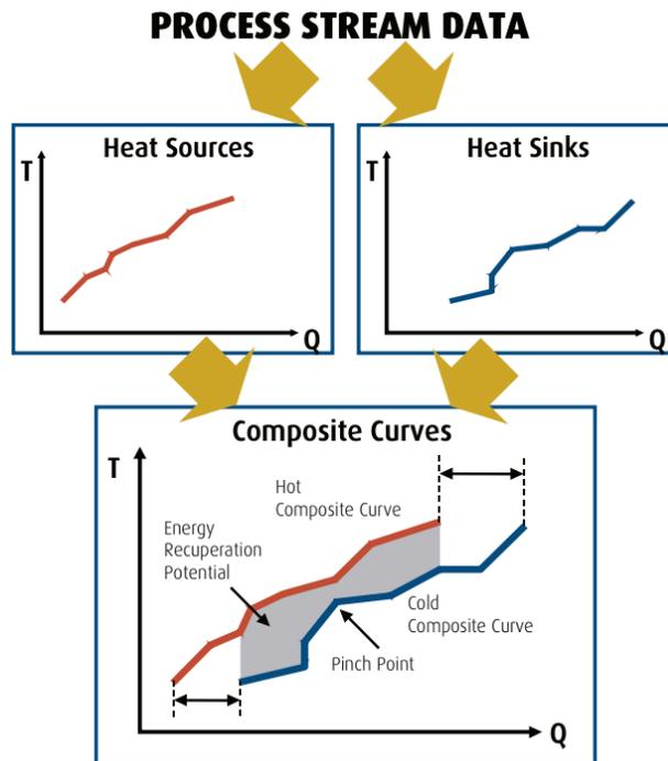
Figure. 8 – Explanation of pinch composite curves (NRCan, 2003)
