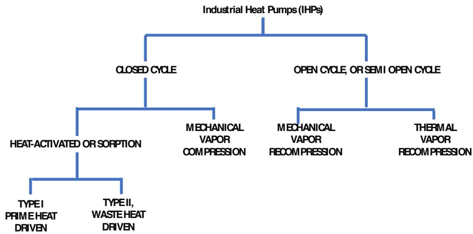
Figure 7 – High level classification of IHP types (EPRI 1988)
