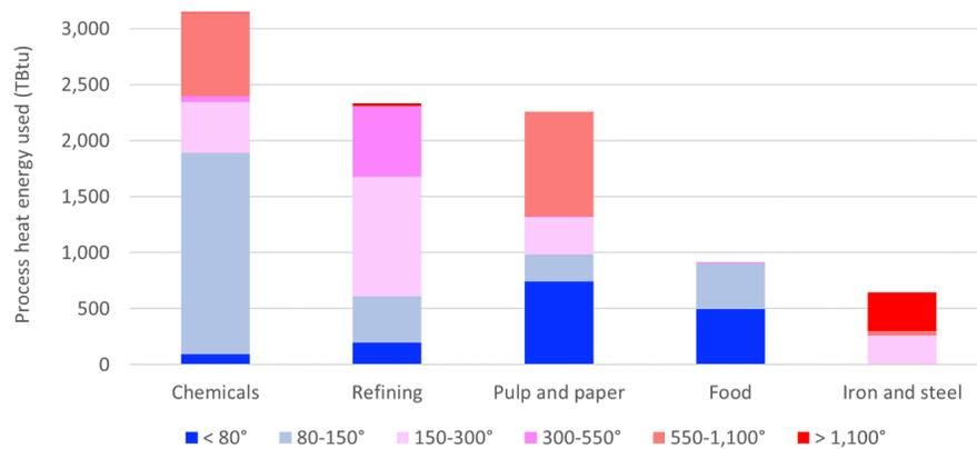
Figure 2 – Process Heat Energy in Industrial Segments. Data Source: McMillan 2019
