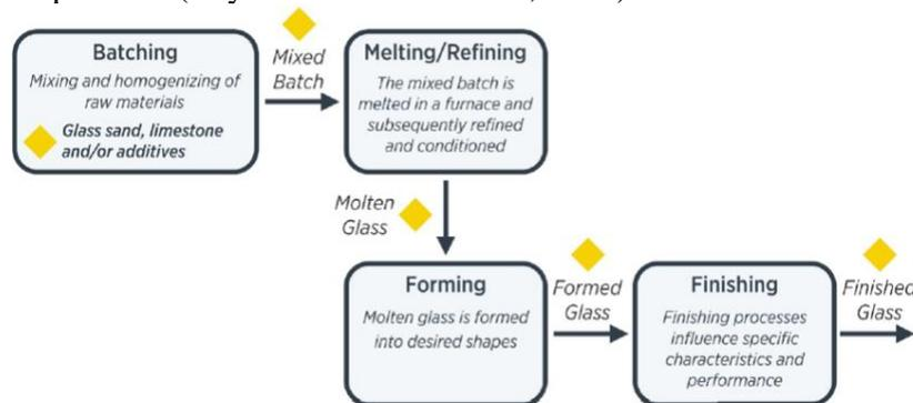
Figure 7. Flow diagram of glass manufacturing (U.S. DOE, 2017a)
