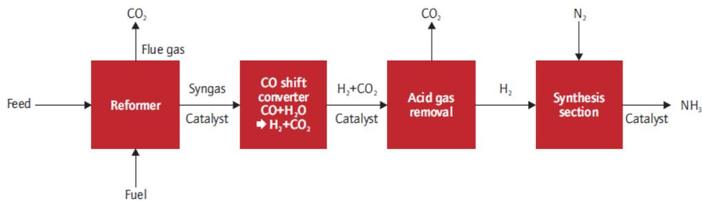
Figure 11. Ammonia synthesis, A simplified schematic
