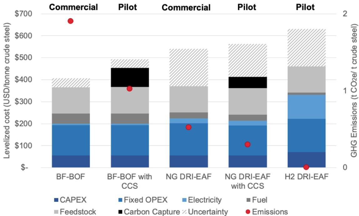
Figure 2. Levelized cost of steel for commercial and pilot routes as greenfield deployments with 3 c/kWh zero-carbon electricity. Emissions include Scope 1, Scope 2, and upstream coking process (Scope 3). *Source:* Own assumptions, based largely on IEA (2019) and Fan and Friedmann (2021). IEA (2019) The Future of Hydrogen, <https://www.iea.org/reports/the-future-of-hydrogen>. All rights reserved.
