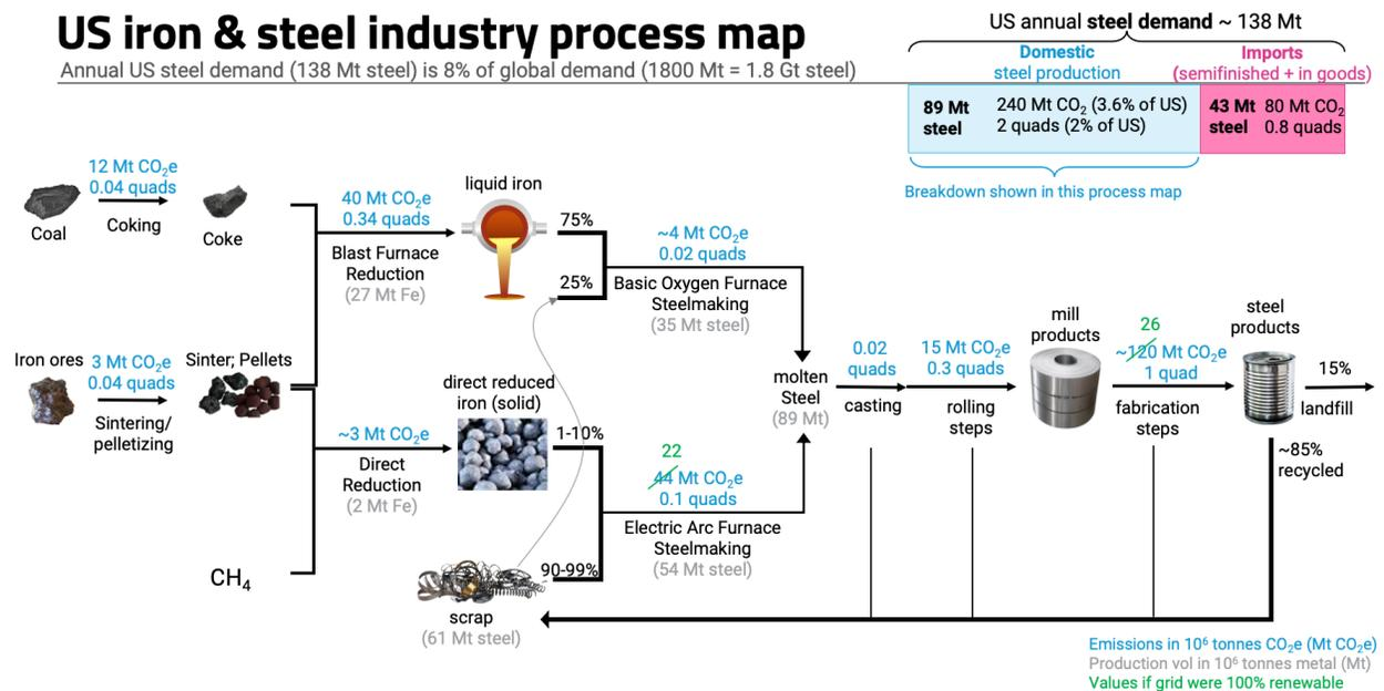
Figure 1. Process map of the United States iron and steel industry annotated with energy use, GHG emissions, and production volumes. These approximate values correspond to the year 2010. *Sources:* World Steel Association 2018; Allwood and Cullen 2015; “Bandwidth Study on Energy Use and Potential Energy Saving Opportunities in U.S. Iron and Steel Manufacturing,”; Fruehan et al. 2000; United States Environmental Protection Agency 2012.
