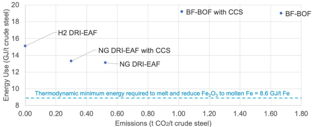
Figure 3. Energy-emissions tradespace for representative commercial and pilot ironmaking routes. *Source:* Own calculations, with assumptions based on values from IEA (2019) and Fan and Friedmann (2021). Thermodynamic minimum energy to produce molten iron is from Fruehan et al. (2000) and is roughly the energy needed to produce molten steel.
