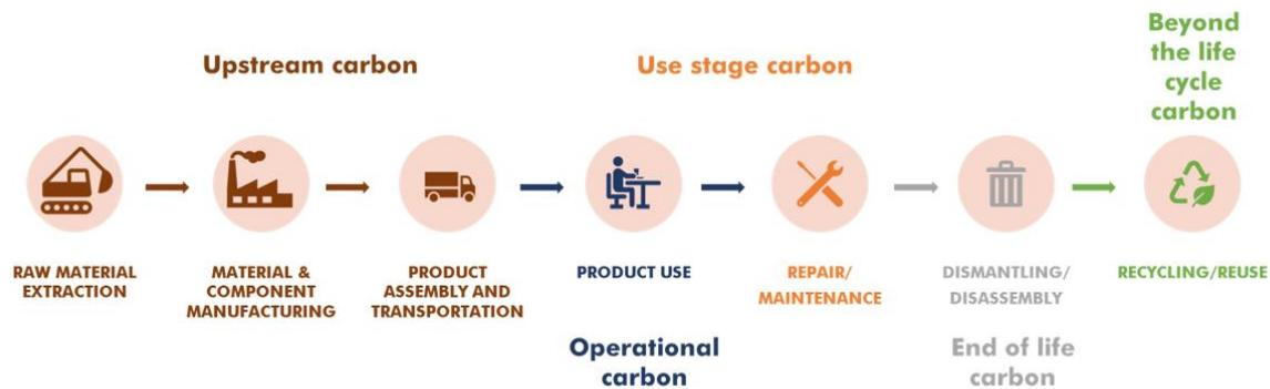
Figure 1. Typical electronic product life cycle. *Source:* GEC 2021b.
