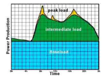
Figure 1. Schematic of base, intermediate and peak load. This shows a typical winter day. Source: Wind Watch 2021. Demand response programs help curtail the need for peak load generation, while energy efficiency programs lower the need for baseload or intermediate load generation.
