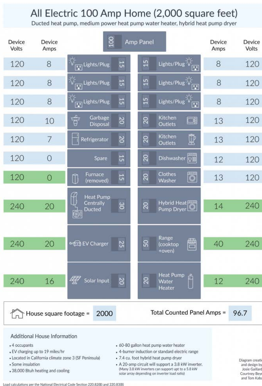
Figure 14. Example of an electrical panel that has undergone a “watt diet” to incorporate multiple circuits on a 100-amp panel. Source: Armstrong et al. 2021.
