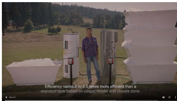
Figure 19. Visual comparison of an efficient heat pump water heater versus a standard tank model. Source: Hot Water Solutions 2021.
