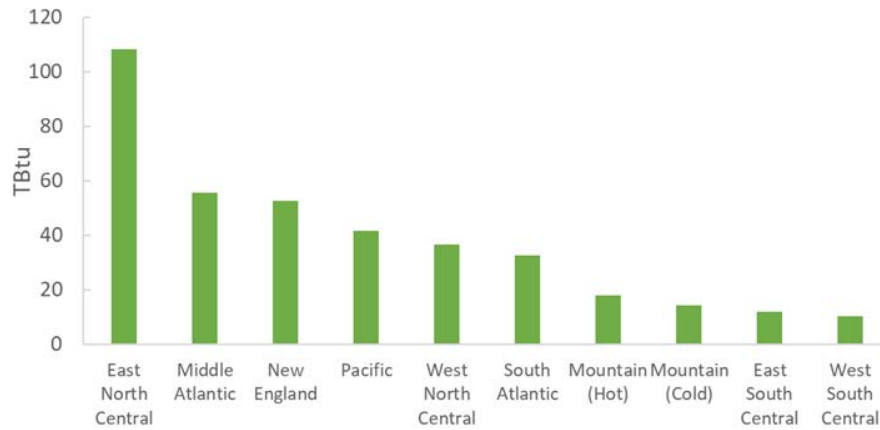
Figure 14. Total energy savings by region from installing a rooftop heat pump when an existing packaged system with gas heat needs to be replaced
