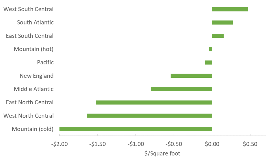
Figure 17. Median lifecycle savings by region for installing a rooftop heat pump when an existing packaged system with gas heat needs to be replaced. This figure does not include the impact of incentives, additional efficiency improvements, or carbon pricing.
