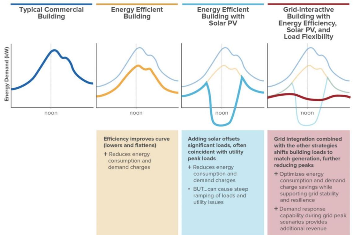
Figure 4. Building load-shape smoothing from efficiency, solar PV, and solar+. *Source:* Carmichael et al. 2019
