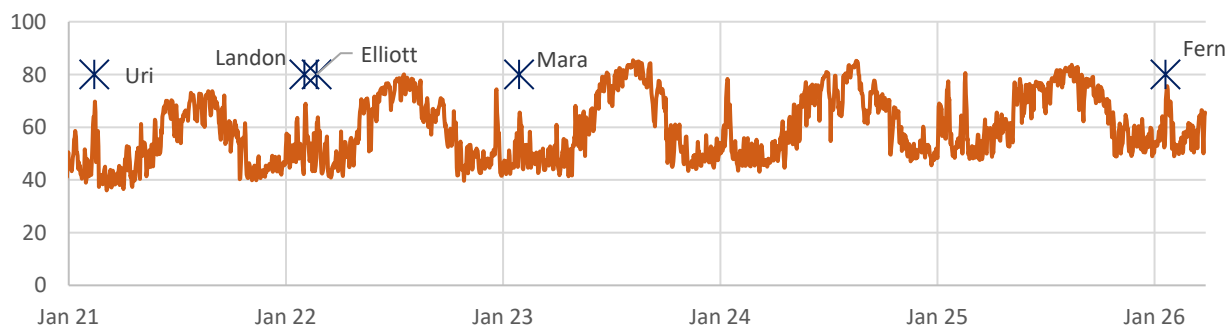
ERCOT Peak Daily Load (GW) January 2021–March 2026 and Beginning Days of Named Winter Storms
