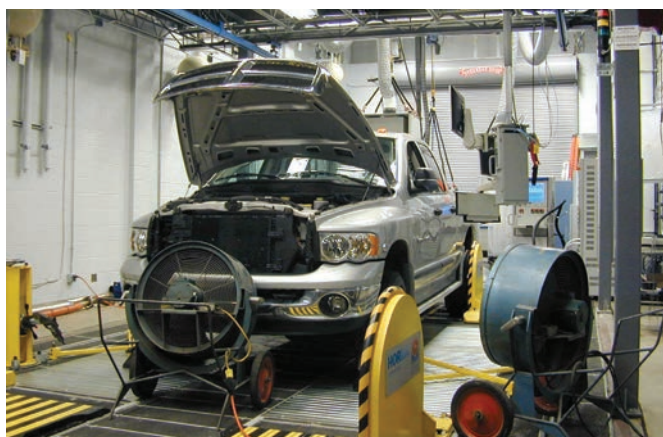
A pickup truck being tested at the National Vehicle and Fuel Emissions Laboratory (source: EPA)
