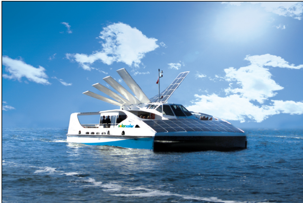
Figure 17: Solar Sailor-Solar/Wind Powered Ferry Currently in Use at the Sydney Harbor and Being Considered for Applications in San Francisco and San Diego
