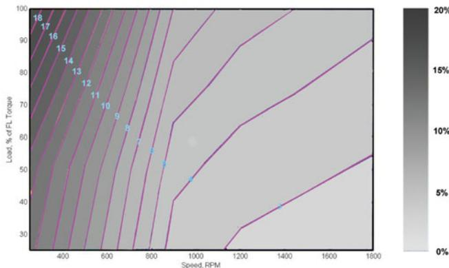
Fig. 8: Efficiency Advantage of PMAC ZEUS Motor™ over NEMA Premium Induction Motor
