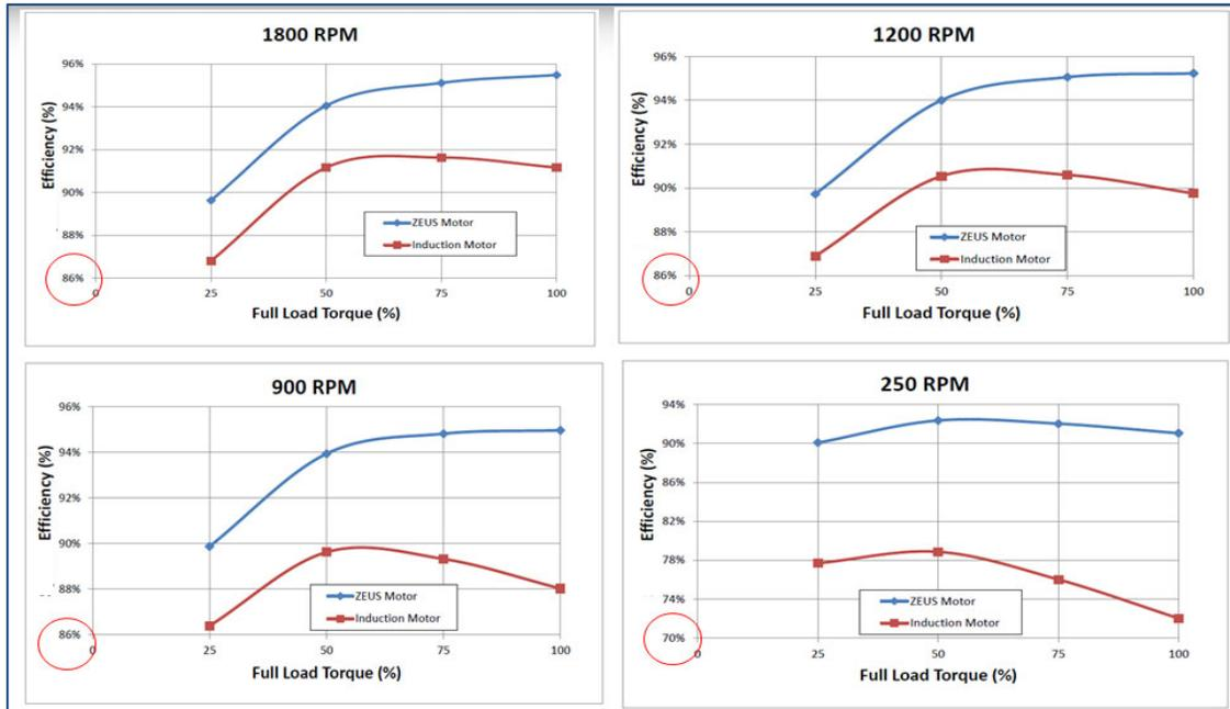
Fig. 6 Motor Efficiency, with VFD
