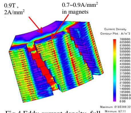
Fig.4 Eddy current density, full load
