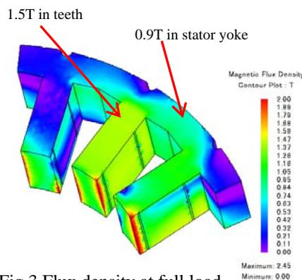
Fig.3 Flux density at full load
