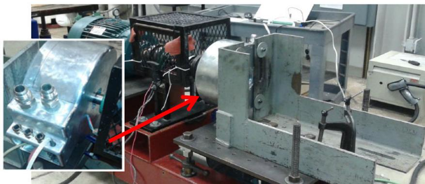
Fig. 5 ZEUS Motor™ under test; TENV cooling, liquid cooling
