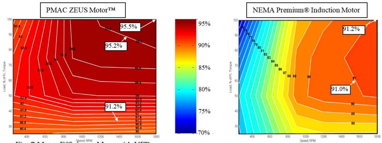
Fig. 7 Motor Efficiency Maps with VFD
