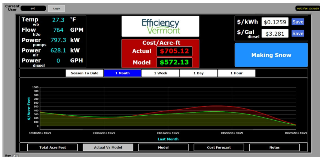
Figure 2. VEIC snowmaking dashboard, displaying inefficient operations across one month.
