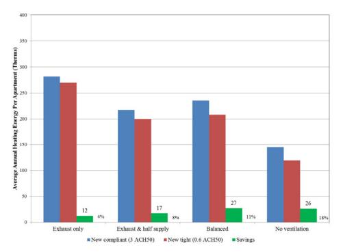
Figure 4: Modelled annual space heating energy use and savings for new construction units
