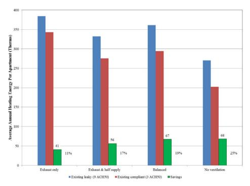
Figure 5: Modelled annual space heating energy use and savings for existing building units
